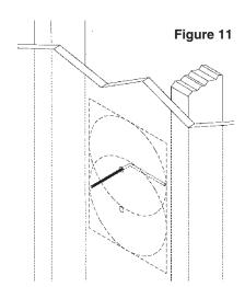
in a complete circle. If it turns freely, repeat the procedure from a hole about an inch above the center of your proposed speaker location (See Figure 11).
